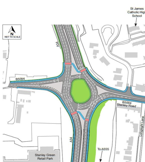
four-arm roundabout joins the A34 and Stanley Road, controlled by traffic lights. Pedestrians and cyclists would be able to cross the A34 in stages using the controlled crossings. This option has two crossing points for pedestrian and cyclists making it a simpler crossing movement.
